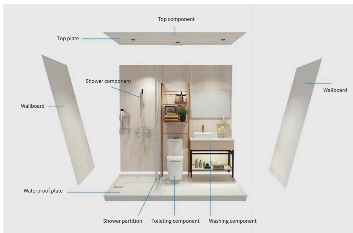
▷ Structure of Assembled Sanitary Ware
