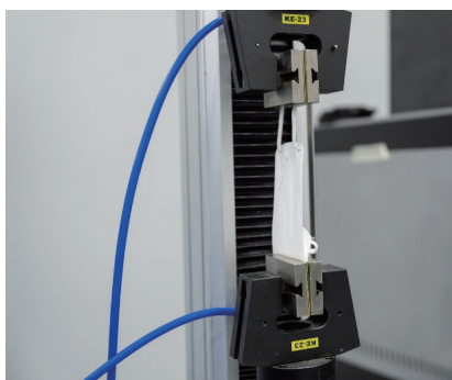
Earloops elongation and weld strength testing
