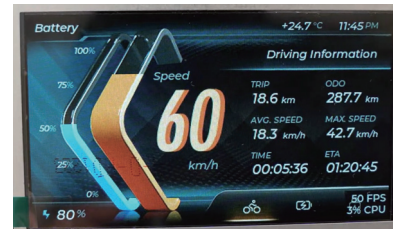
A 4.3-inch LCD screen functioning as a dashboard connected to our AiPi-SPC-4.3 board
