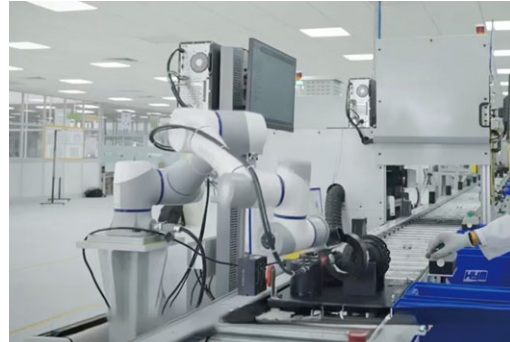
Wheel hub motor testing
