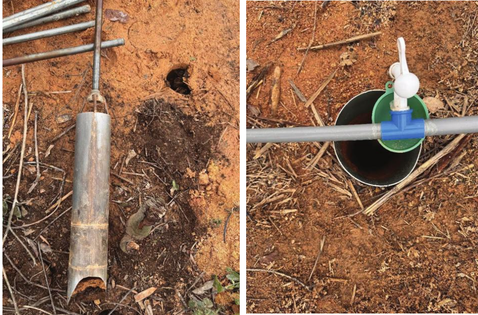
Figure 12-6: Auger and Injection Hole
