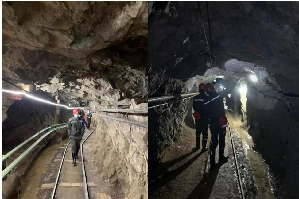
Figure 10-7: Photos of Typical Level Drift and Cross Cut Drift of Lianhuagou #5 Zone
