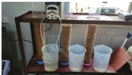
Figure 9-1: Laboratory Leaching Test
