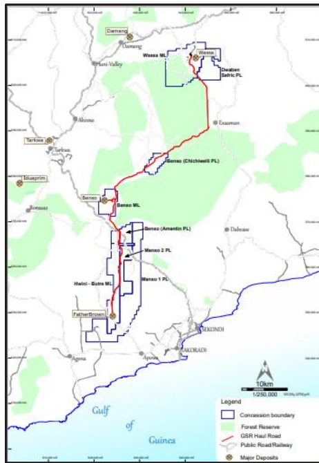
Figure 7-1: Layout of GSWL Mining Leases and Prospecting Licences Linked by Laterite Sheeted Haul Road
