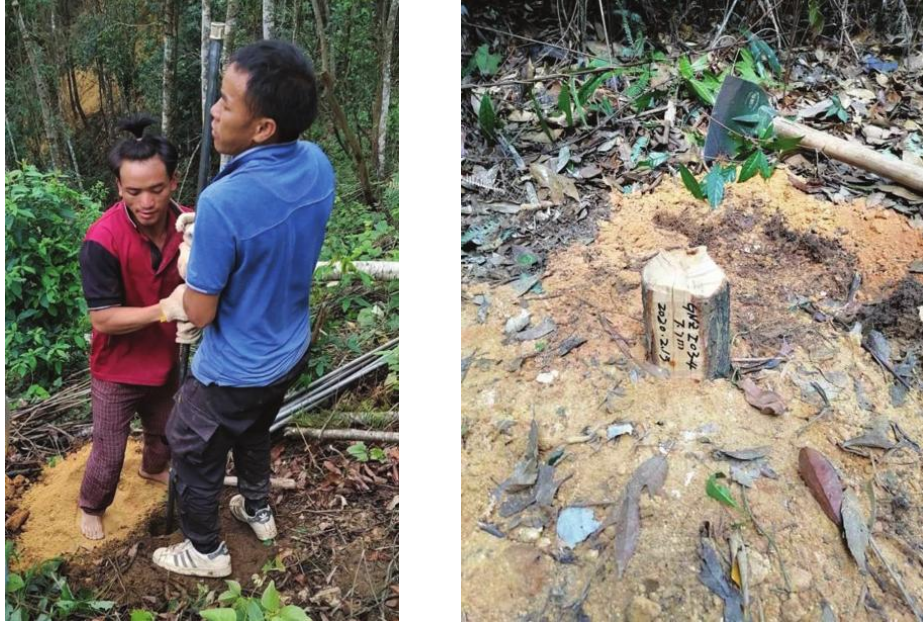
Figure 7-3: The GN Auger Utilization and Hole Sealing
