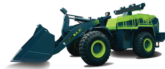
BRT958KLe, our first cabinless remote-operated loader
