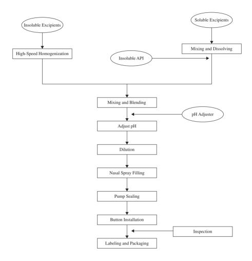
For nasal sprays, in addition to maintaining particle stability, the manufacturing process requires the addition of a suspension aid, which imposes greater demands on the sequence of material addition. Utilizing our proprietary inhalation formulation technologies, we have been able to maintain consistent particle stability throughout the manufacturing process.
