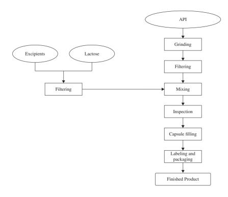
The manufacturing of DPI products involves a combination of drug and devices. In addition to maintaining particle stability, it is also important to design and develop a suitable delivery device. We have successfully designed and developed our proprietary delivery device for our powder inhalation formulation products, which we believe is well-suited for the APIs we use and can enhance the stability of our powder inhalation products.
