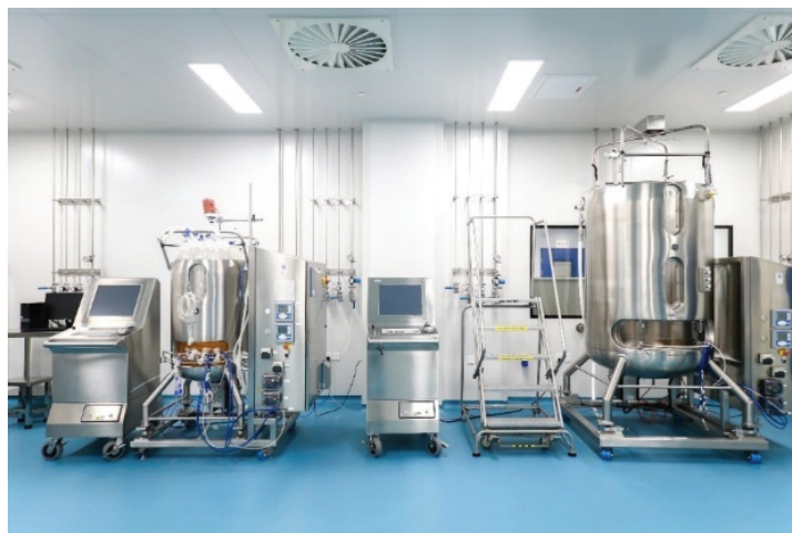
Our 200L and 1,000L drug substance production line for CHO
