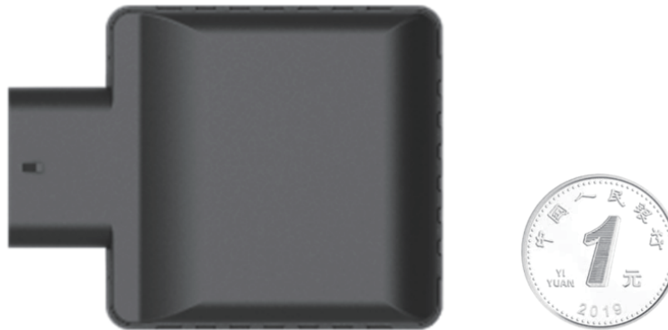
CTMRR-410 radar – body size of only 55 mm × 53 mm × 16 mm
