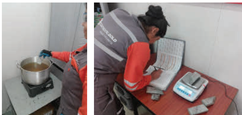
Figure 6-6: Sample Dipped in Paraffin and Sample Weighing
