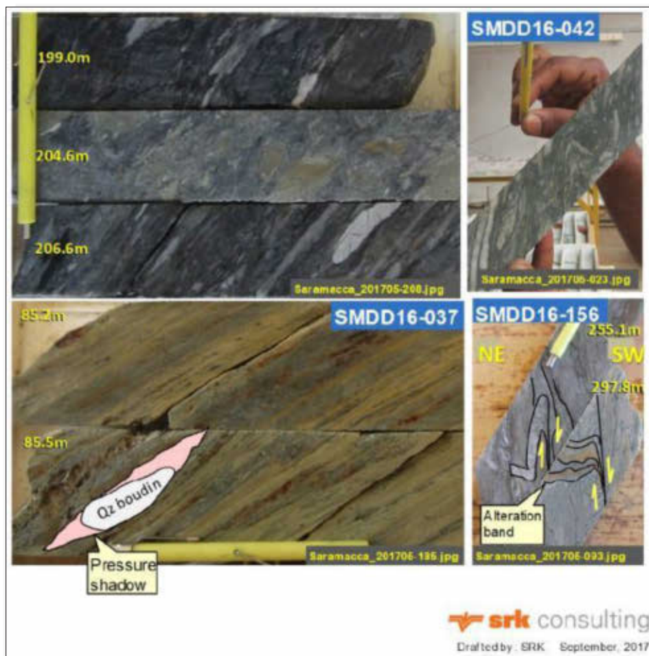
Figure 5-4: Example of Typical Ductile Features, Faya Bergi Fault (SRK, 2017A)
