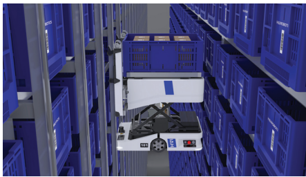
Step 1: Climbing and retrieving a case from a designated rack
