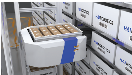
Step 1: Picking a case (without moving the entire rack)
