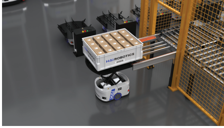
Step 3: Transporting the case to a designated workstation
