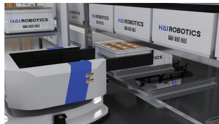
Step 2: Transporting the case to AMRs
