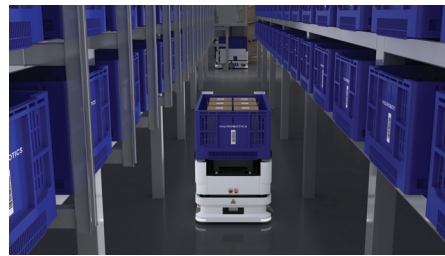
Step 2: Transporting the case to a designated workstation
