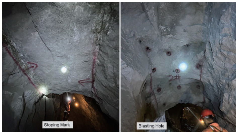
Figure 16.8: Stopping Management and Blasting Holes
