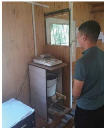
Figure 11.4: SG Measurement of Core Sample from Kyzyltash in 2021
