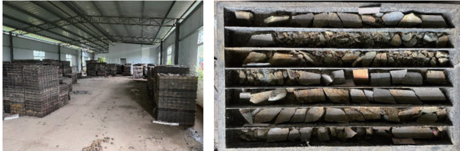
Figure 10.4: Core Storage Room and Core Boxes
