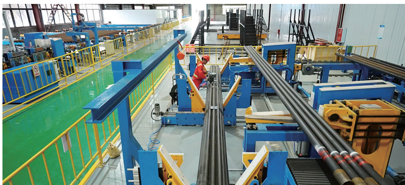
Conduct inspection and repair for casing and tubing
