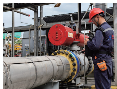
Performing leak detection with portable helium leak detector at production station
