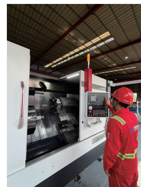
Performing precision machining of casing and tubing pub joints
