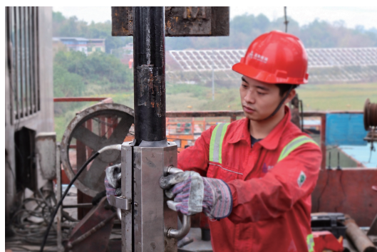
Conducting gas leak detection for downhole tubing at drilling platform
