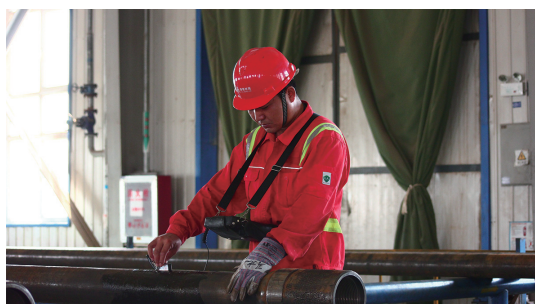
Carrying out ultrasonic testing on drilling tools
