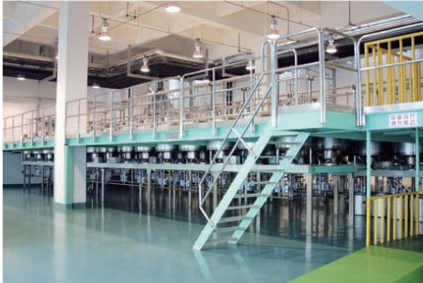
Casing and flavouring system equipped with storage, retrieval and feeding devices
