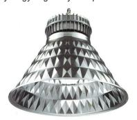
This series of product uses a circle tube as its light source with an optional aluminium lamp reflector, mirror-like polishing. A specific model of this series has an ultraviolet anti-ageing silicon gasket. It is available in different wattages and different colour temperatures. Its applications include warehouse, car park, repair and maintenance centre, factory and supermarket.
