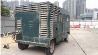
Air compressor is mainly used for removing the excavated material by air lifting method from drilling and shotcreting operations
