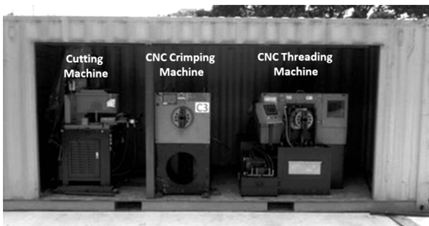
Three types of mechanical splicing machines located at workshops
