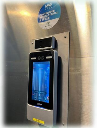
Caption: Access Controller with temperature measurement 圖片說明：探熱測溫門禁系統
