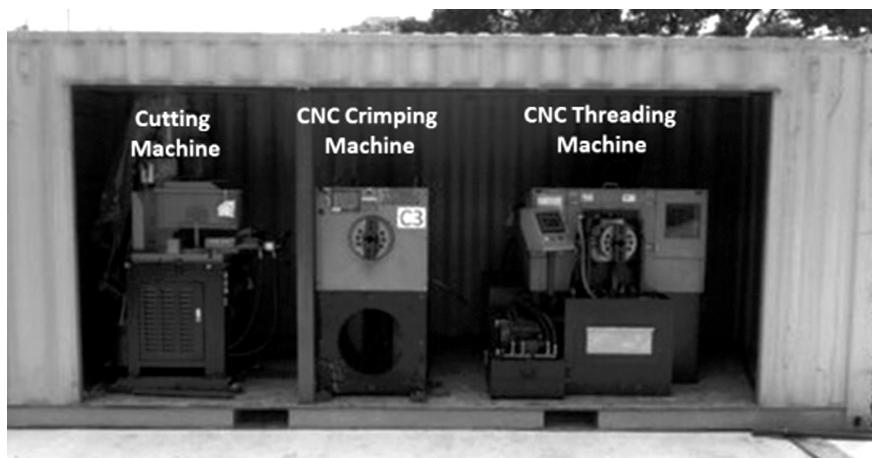
Three types of mechanical splicing machines are located in workshops
