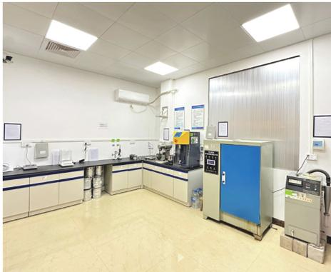
Used for conducting physical performance tests and evaluating the performance indicators of cement, which include testing standard consistency water requirement, stability, initial and final setting time, and strength of the samples and collaborating with other departments for related experiments.
