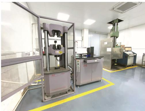
Used for testing the mechanical properties of metal materials, which includes inspecting the appearance dimensions and weight deviations of the materials, conducting tensile tests to measure the material's strength, and evaluating the material's yield strength and bending performance.
