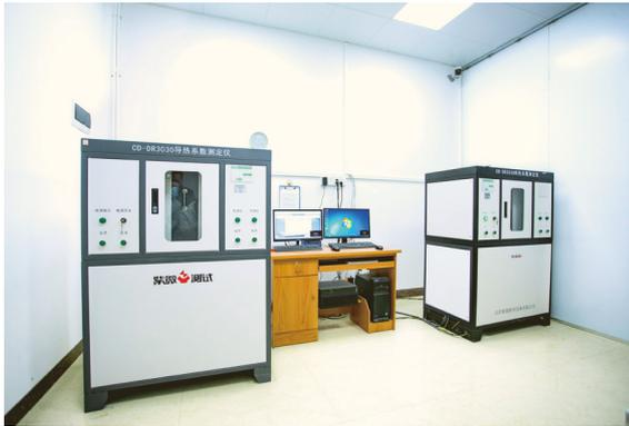
Used for testing insulation materials, which includes testing the thermal insulation mortar for building insulation, thermal conductivity of insulation materials, thermal conductivity of extruded polystyrene foam for insulation purposes, thermal conductivity of autoclaved aerated concrete blocks, and dimensional measurements.
