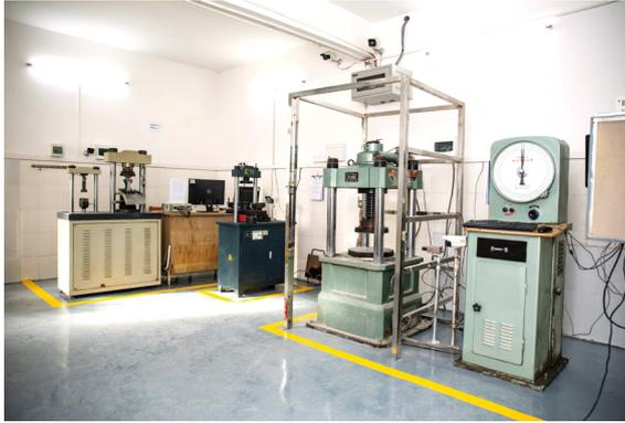
Used for evaluating the mechanical properties of non-metallic materials, which includes testing the compressive and flexural strength of concrete, mortar, wall materials, pavement bricks, and curb stones.
