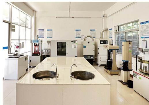
Used for conducting physical and chemical performance testing, performance indicator evaluation, and mix design of asphalt mixtures. The main testing include compacting asphalt mixture density, theoretical maximum relative density, stability and flow value, dynamic stability, permeability coefficient, saturation rate, asphalt mixture aggregate gradation inspection and strength testing.
