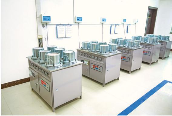
Used for conducting testing on the permeability of concrete, which includes measuring the water permeability of concrete.
