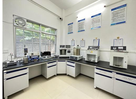
Used for conducting physical and chemical performance tests and performance indicator evaluations for various types of asphalt, which include but are not limited to: asphalt penetration degree, softening point, elongation, density and relative density, wax content, flash point and ignition point, dynamic viscosity, standard viscosity, kinematic viscosity, emulsified asphalt residue, emulsified asphalt particle ion charge, emulsified asphalt storage stability, and demulsification rate testing.
