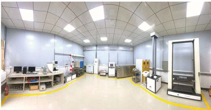
Used for testing plastic pipes, including single-material plastic pipes such as rigid polyvinyl chloride (PVC) pipes, polyethylene pipes, polyethylene pipes, and PVC plastic pipes.
