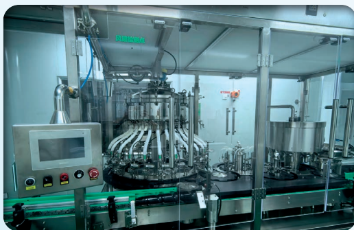
Filling, nitrogen charging and stoppering machine
