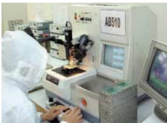
線路版鑲芯片焊線工藝 Chip-On-board assembly process
