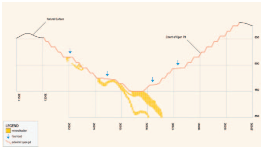
Figure 5-3: Schematic Section Through Open-pit (Matrix Consulting, 2004)
