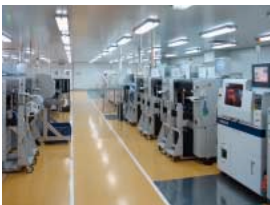
在無塵車間操作的先進電路板貼裝設備 Advance SMT Lines in clean room working environment
