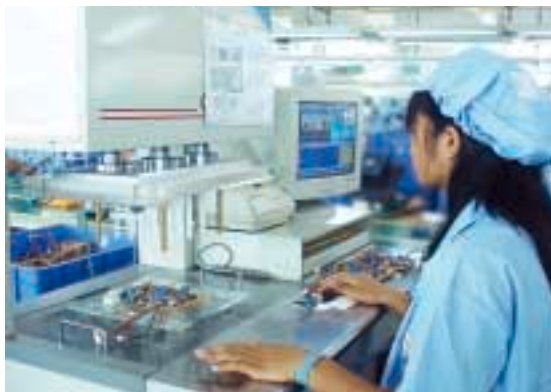
電路板經在電路測試系統檢定後才投入整機裝配生產 In-Circuit Testing System ensuring good PCBs applied to final assembly process
