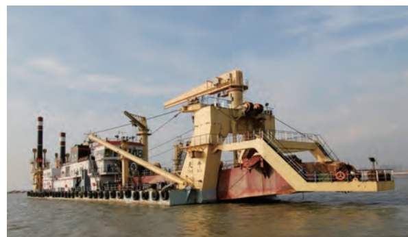
"Tian Niu", the largest cutter suction dredger in China
