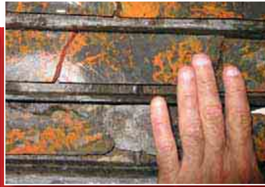
Jinfeng drill core with orpiment veining
