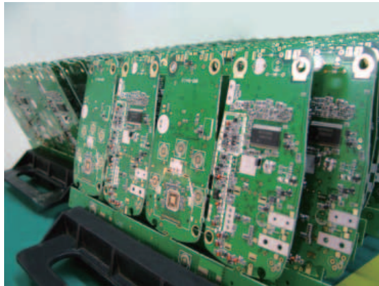
我司電子製品之新發展，圖中的為對講機的半成品電路板 Walkie-Talkie PCBs, a new market sector being develop for the consumer electronics manufacturing business
