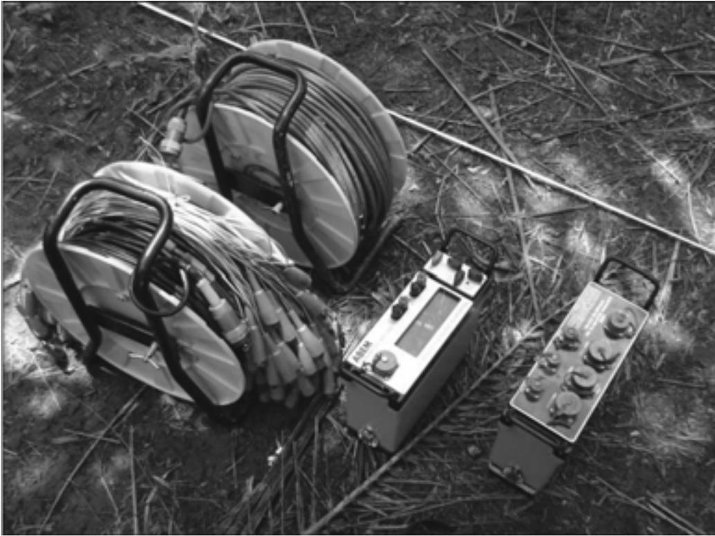
**Fig. 17:** The instrumentations for geoelectrical resistivity imaging survey.
