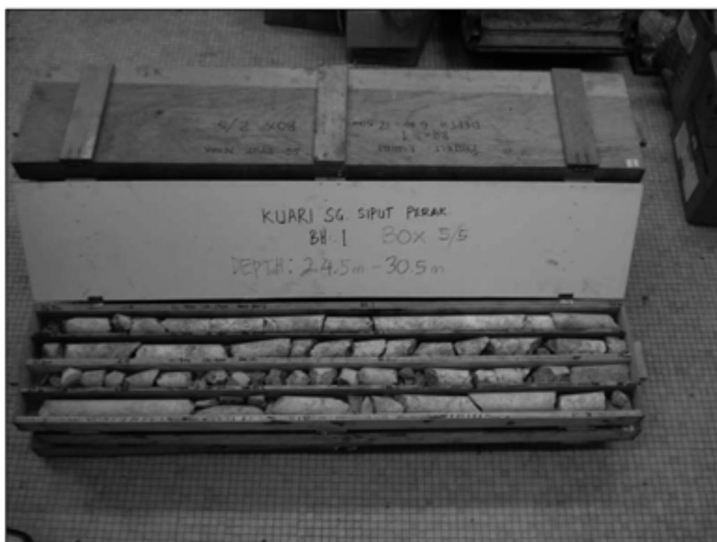
**Fig. 13:** The core samples from the drilling conducted at BH-1 (the South Hill).
