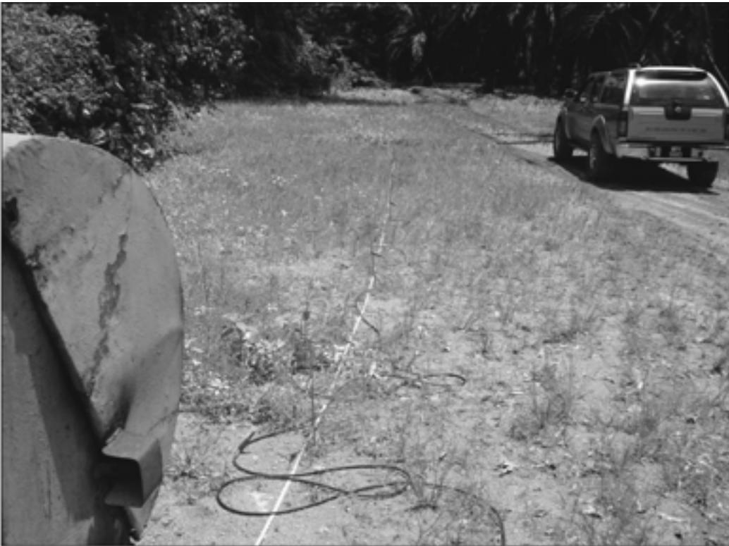
**Fig. 18:** The geophones on the geophysical traverse line at the vicinity of the North Hill.
