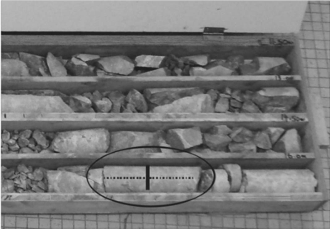
**Fig. 14:** The close-up of borehole samples with the marked area to be pulverized (BH-1; South Hill)
