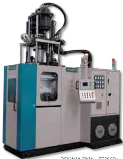
DEKUMA DKM – RT280Sv 伺服驅動節能橡膠注射成型機
