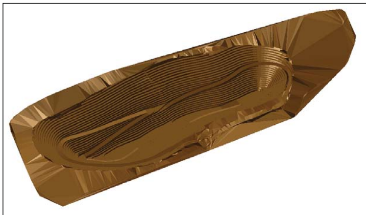
Figure 20: T-17 Open Pit Final Design
