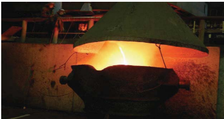
Photo 16.1: Tapping Lead Bullion from Lead Blast Furnace
