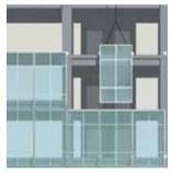
A unitized curtain wall is another type of frame-supporting curtain wall consisting of framing components and panel materials. Such framing components and panel materials are assembled into a single curtain wall unit at our production base. The curtain wall units are then transported to construction sites for installation. The panels can be made of various materials, including glass, metal, stone, and artificial materials.
