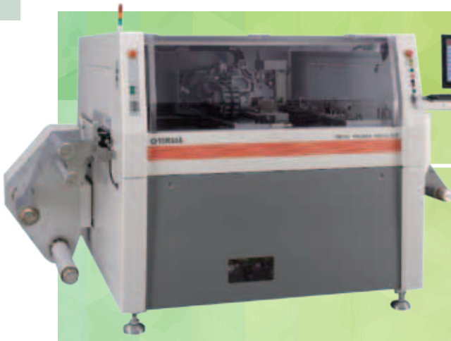
Yamaha MR512GFR Reel to Reel Micro Prober Yamaha MR512GFR 卷對卷電測機
