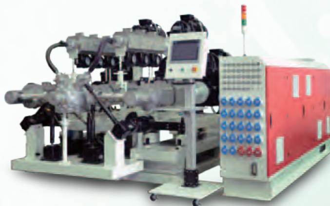
Multilayer Nylon Composite Pipe High-speed Extrusion Line 多層尼龍複合管生產線
