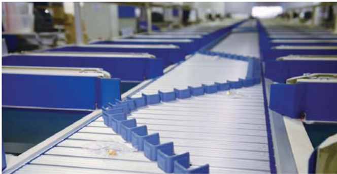
RFID-embedded sorter can automatically sort the products to the designated POS 結合RFID技術的輸送帶可自動分揀貨品到指定的零售點
