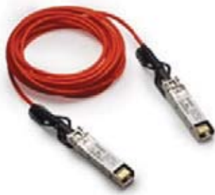
Active Optical Cable – 25G Ethernet
