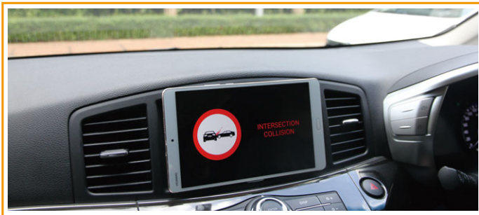
An alert will be issued when two vehicles are approaching the same intersection point.
