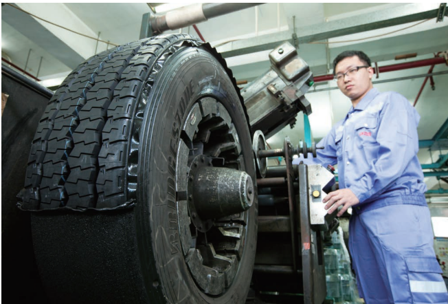
KMB and LWB tyres are retreaded to reduce solid waste disposal 為減少固體廢物，九巴及龍運進行輪胎翻新
