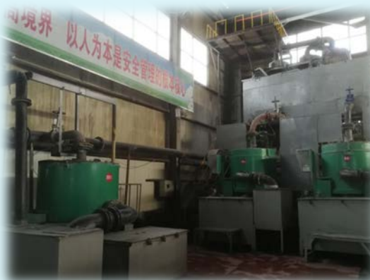
Dust removal system at crushing section after reconstruction
