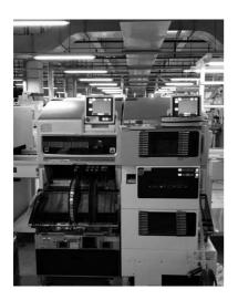
The automated mounters pick up components including chips, ICs, connectors by vacuum placement heads and place them on the PCB. Mounting time per chip ranges from 0.1 second to 0.3 second with high precision ranging from 0.01 mm to 0.05 mm. After placement, we will conduct visual inspection to check if components are properly placed according to our customer's requirements or product specifications.
