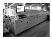
After mounting, PCB is transferred by conveyor belt to pass through a re-flow oven for soldering the components. In the reflow oven, solder paste applied on the board is heated and melted to keep the IC in place, and then the molten solder paste is cooled to keep the IC attached to the PCB. This step is to solidify and adhere the electronic components onto the PCB.
