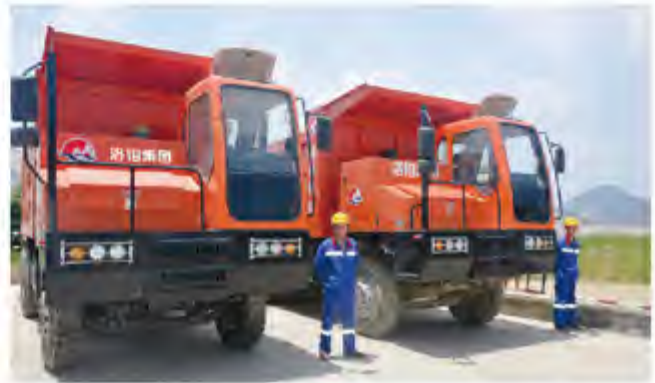
In 2018, we have successfully developed electric driverless mine truck operations, which have passed the inspection of the National Mining Machinery Quality Supervision and Inspection Center. Radar, camera, and sensors provide multiple omnidirectional sensing, vision-based target detection and recognition and moving target trajectory. Under this system the truck can plan a route and give feedback in real time so that automatic driving can be realized, driving safety can be improved and the occurrence of casualties can be reduced.
