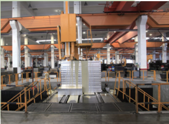
立式帶鋸將鋼材鍛件切成粗形 Vertical band saws cut steel blocks into rough shape
