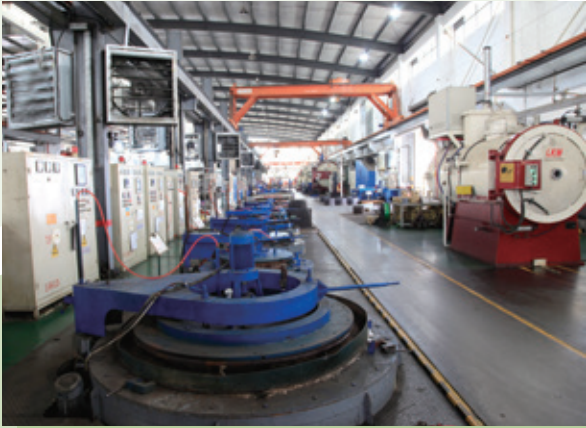
真空熱處理爐及井式回火爐提供穩定的熱處理加工服務 Vacuum furnaces and vertical tempering furnaces provide stable heat treatment services
