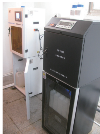
Treated waste water monitoring system
