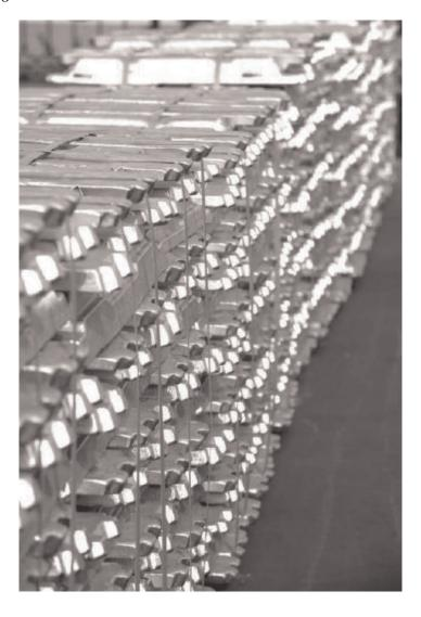
Sales of aluminum alloy ingots accounted for approximately 12.0% and 4.5% of our revenue for 2017 and 2018, respectively. Molten aluminum alloy is processed into aluminum alloy ingots through molding, casting and cooling. Our aluminum alloy ingots are produced by using self-manufactured molten aluminum alloy.
