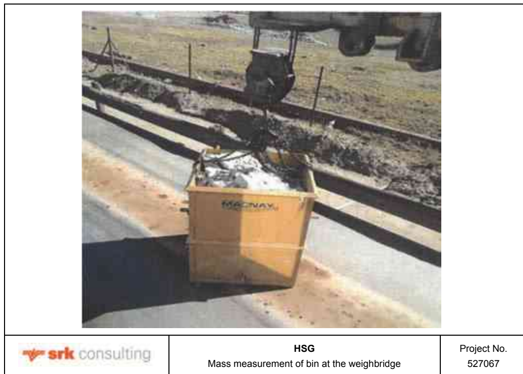
Figure 6.3: Image of one of the sample bins being weighed at the Nicolor Plant weighbridge
