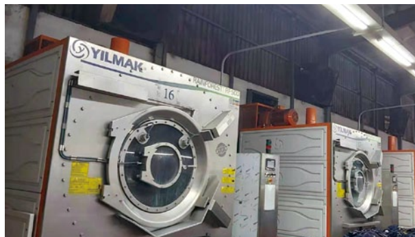
Texhong Thai Binh Garment: water-saving washing machines 天虹太平服裝：節水洗衣機
