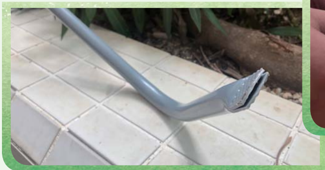
The devised hose with a narrower pipe outlet 改裝後管道變窄的喉管
