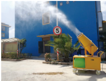
Picture of an operating fog cannon 霧炮機工作畫面
